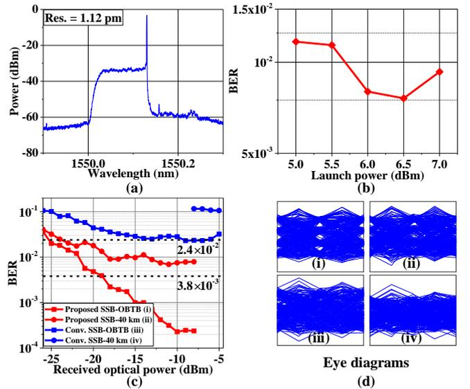
Fig. 4. (a) Optical spectrum of the generated SSB signal. (b) BER versus launch power. (c) BER curves for the OBTB case and after the 40-km SMF transmission. (d) Eye diagrams in the different cases.
