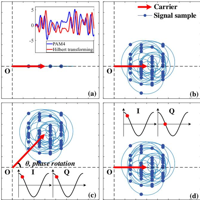
Fig. 1. Time trajectories of (a) a DSB-PAM4 signal, (b) a VSB-PAM4 signal, (c) a conventional H-SSB PAM4 signal, and (d) a proposed H-SSB PAM4 signal, respectively. Inset: baseband PAM4 signal and its Hilbert transform.
